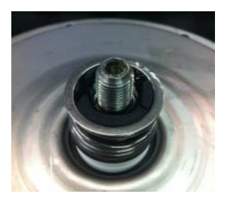
3.10 Press the rotating half down evenly until its face meets the stationary face. The spring will compress, and as you let go will slowly rebound. The top of the seal should be slightly above the shoulder on the shaft. Do not press the top of the rotating seal past the shaft shoulder
