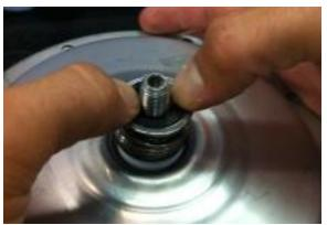
3.11 After installing the seal, screw the impeller onto the shaft until it stops at the shoulder on the motor shaft. You may need to prevent the motor shaft from rotating by inserting a screwdriver into the slot, found in the rear/center of the motor.
