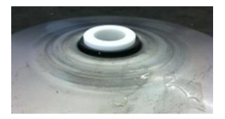
3.05 Press the stationary seal into the sealplate , using the butt of the screwdriver to find the center. The seat must be all the way against the sealplate bore.
