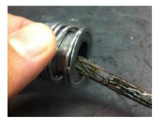
3.09 Carefully slide the rotating half over the motor shaft without damaging the seal face.
