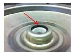
3.07 Install the sealplate and stationary seal onto the pump carefully. Do not damage the face of the stationary seal when installing over the motor shaft.
