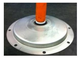
3.06 Turn the sealplate upside down. Check to ensure the seal seat is pressed all the way against the sealplate bore. If it is not, you will see a gap between the rubber elastomer and the sealplate.
