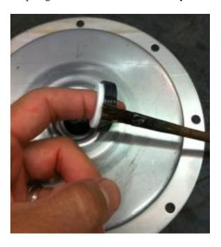
3.04 Set the stationary half of the seal into the seat as level as possible.
