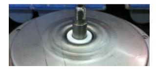
3.08 Lubricate the rubber in the inner diameter of the rotating seal half with the brush.
