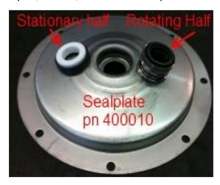
3.03 Apply soapy water (see tools required) to the outside of the seat on the stationary half of the seal. Do not let the liquid get on the face of the stationary seal
