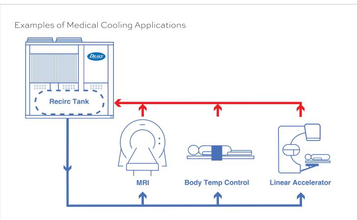
Critical temperature tolerances are difficult to maintain under varying conditions. Drake recirculation tanks can hold temps to +/- 1°F.
